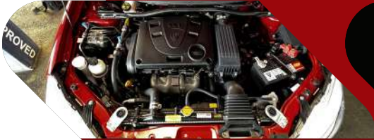
1.3L, 4 Cylinders In-Line, 16 Valve DOHC, VVT Engine
