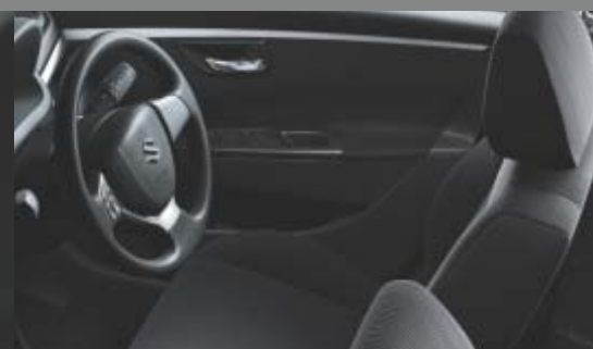
TILT STEERING AND DRIVER SEAT HEIGHT ADJUSTMENT
