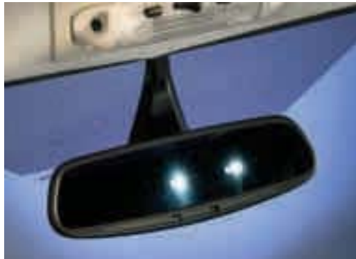
Auto-dimming rear-view mirror Helps take the glare away from reflected lights. (Standard)
