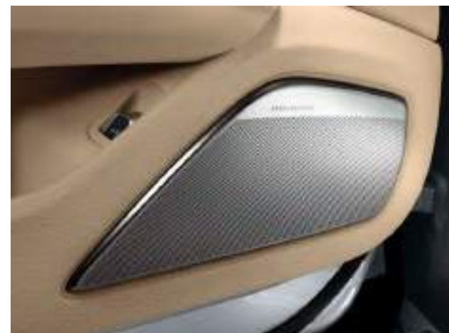
Bang & Olufsen® Advanced Sound System with 19 speakers and 1,400 watts (optional on TDI®, 4.0T and W12 models)
